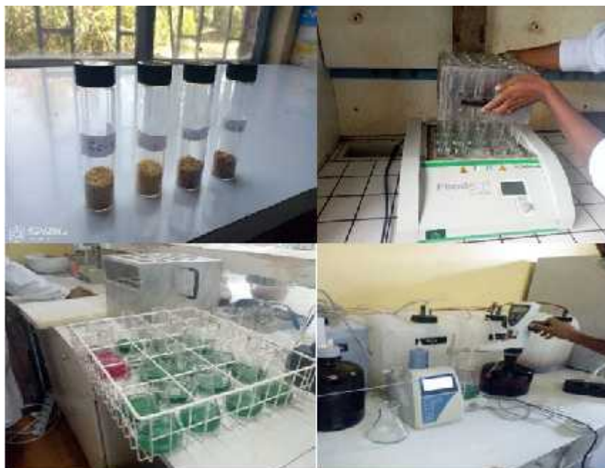
Fig. 21: Sample preparations: Clockwise: Digestion, distillation, titration and Nitrogen content determination of B. carinata using Kjeldahl method
