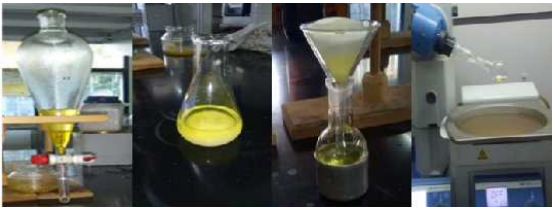
Fig. 20: Left to right: Left to right: Drying with anhydrous \text{Na}_2\text{SO}_4 , Filtration and Concentrating by rotavapour
