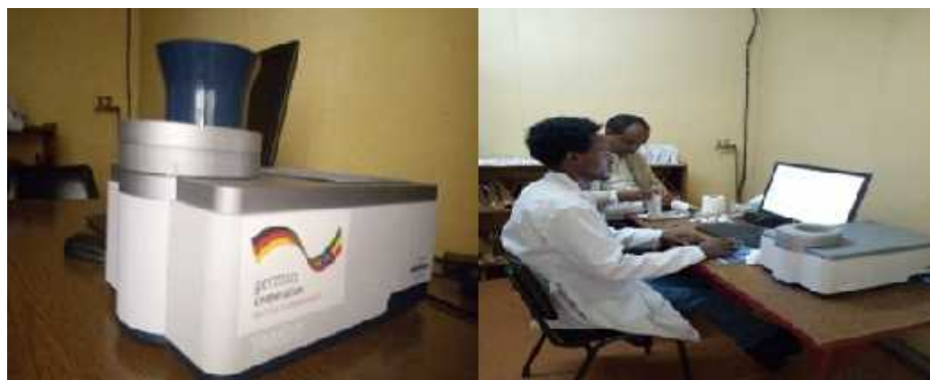
Fig. 22: Spectra collection of B. carinata samples using Tango-Bruker FT-NIR
